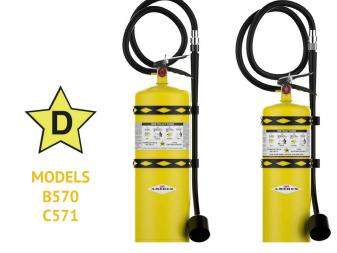
MODEL B570 contains a special blended Sodium Chloride-based dry powder extinguishing agent. Heat from the fire causes it to cake and form a crust excluding air and dissipating heat from burning metal. Metal fires involving magnesium, sodium, potassium, and sodium-potassium alloys can be successfully extinguished with this extinguisher. There is data showing that zirconium, uranium, titanium, and powdered aluminum fires can be controlled and extinguished with this unique extinguisher.
